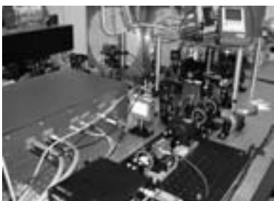
Fig. 2: The injection locked laser system for GEO600 (lab system)
